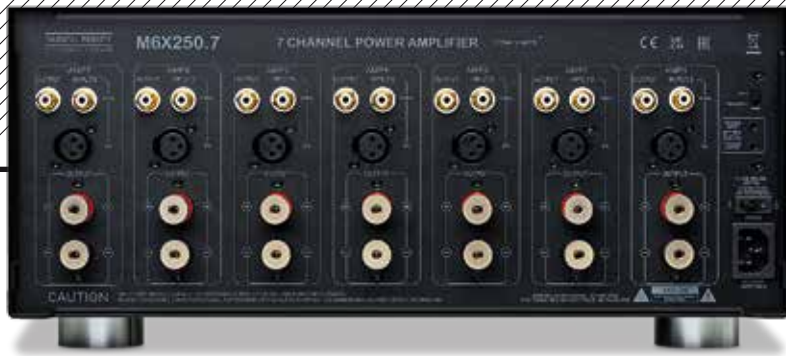
ABOVE: Seven separate amplifier modules are accessed from the rear panel, each with (unswitched) RCA and XLR inputs, a daisy-chain line output on RCA and speaker connection on 4mm posts. Auto signal sensing and 12V trigger control is included
